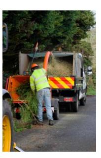
The knife blade caught the corner of the hood, throwing the hood into the impeller. The hood was blown off the chipper and fatally struck the worker in the chest.
