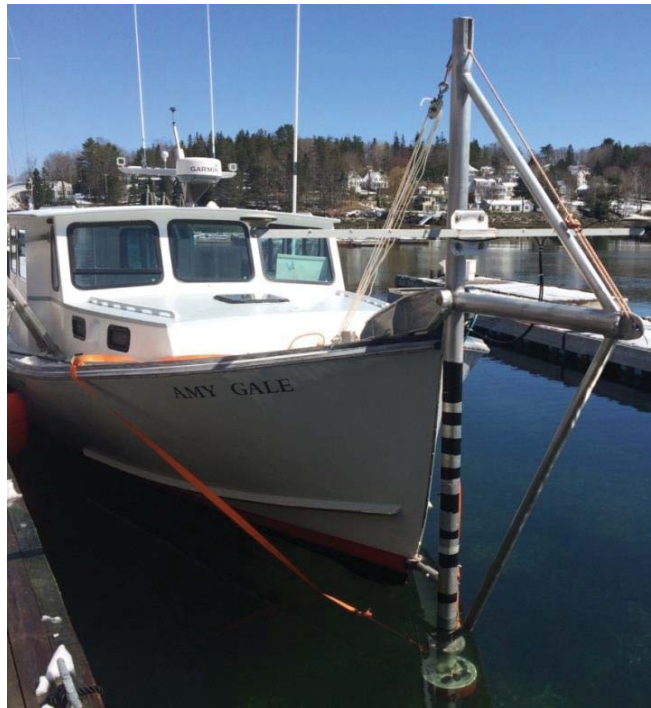
Figure 3 – R/V Amy Gale shown with pole-mounted dual GPS antennas, Kongsberg EM2040c multibeam sonar, MRU (not visible), and surface sound speed probe (not visible) in acquisition mode
