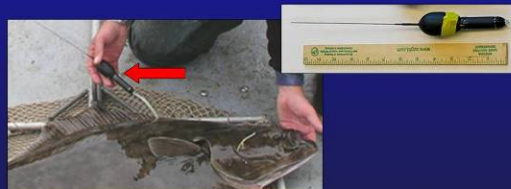
Figure 3: Atlantic halibut with PSAT, tether and conventional tag, to the right is PSAT tag with magnet.
