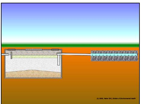
Primary treatment, which takes place in the treatment tank, is a settling process in which the settleable solids sink to the bottom by gravitation and lighter elements float to the top.
