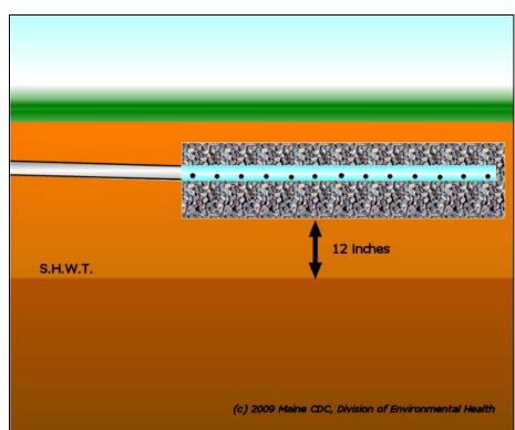
The movement of septic tank effluent through the biomat is due to the hydrostatic or gravity head pushing the septic tank effluent down through the biomat, and the capillary tension force or matrix potential pulling the septic tank effluent through the biomat. In many soils the capillary potential of the soil itself is more effective than the small hydrostatic heads in forcing the septic tank effluent through the biomat.
