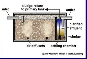
The primary advantage of aerobic treatment is that the low nutrient, high D.O. effluent requires a much smaller disposal area. In many cases, the disposal area size can be reduced by as much as 50%.
