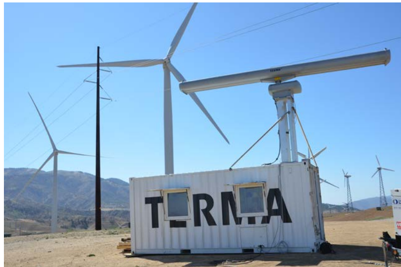
Figure 6. Terma SCANTER 5202 PSR Installed at TWRA
