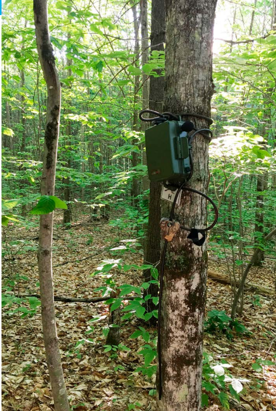
The battery-powered songmeters can record for hundreds of hours.
