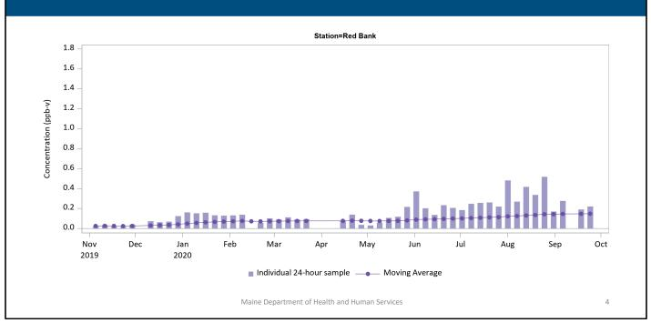
Bar height reflects concentration of chemical measured in a 24-hour sample collection. The line and circle markers show the cumulative average at a point in time. The final circle marker shows the cumulative average from the prior 11 months of sample results.
