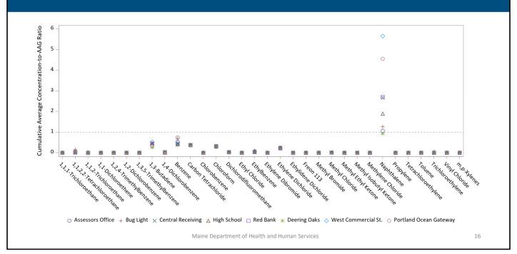
This figure shows the result of comparing all cumulative averages for all the 24-hour sampling results to their corresponding AAGs for those chemicals where we have an AAG. A ratio of 1 means the measured level is at the AAG. A ratio of less than 1 means the measured level is below the AAG. Naphthalene and acrolein (next figure) are the only chemicals that had cumulative averages above their corresponding AAG.
