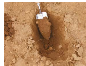
Insert the trowel again ½ inch from the first cut and just as deep. Collect a thin slice of soil, and place it in a clean bucket.
