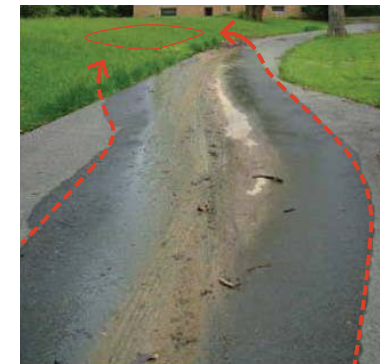
Make observations after a rainstorm to determine the direction of the runoff and the drainage area of the rain garden.
