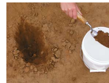
Repeat this procedure about ten times, and combine all of these soil cores into one composite sample.
