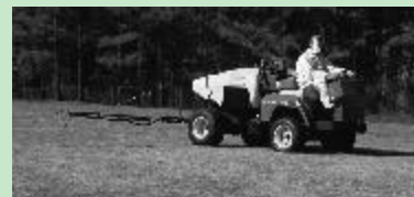
Figure 2. Determine miles per hour by driving the sprayer through a 200-foot course.
