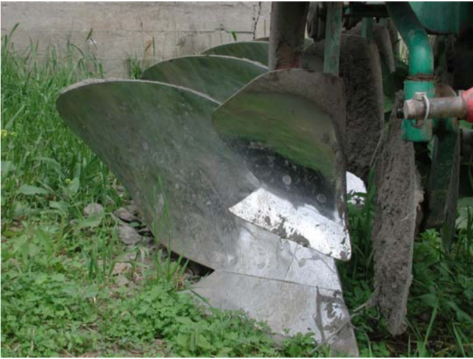
Figure 10 – The skim coulters on a plough helps to bury quackgrass rhizomes and stems in the bottom of the furrow more effectively.
