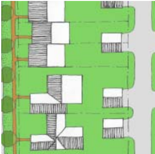
A. Mixing duplexes and townhouses within the same block creates higher density. The duplexes sit on 6,000 SF lots. The townhouse 'lots' are smaller at 3,600 SF each. In both cases the units have garages accessed off an alley. The garages can be either attached or detached.
