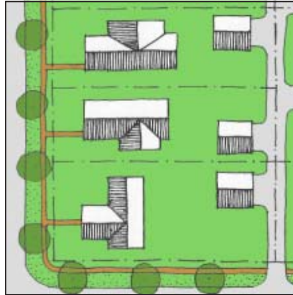
A. 3 single family homes on 3 lots totalling 1/2 acre: 6 dwelling units per net residential acre. Lots are variable in size: corner lot is 8,900 SF, the others are 7,000 SF.
