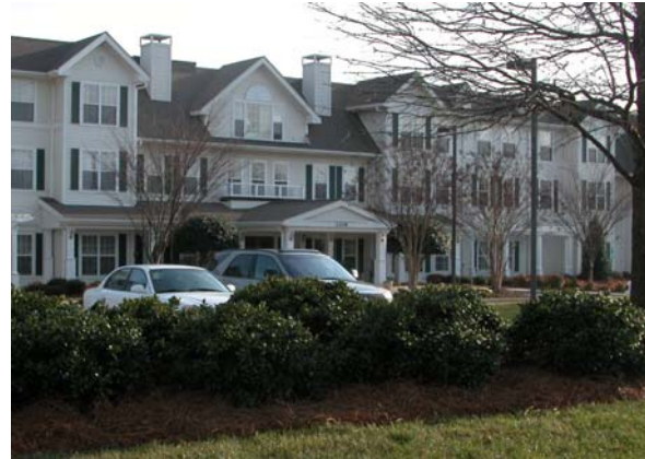
Trees and shrubs on a low mound effectively screen this parking area from the public road.
