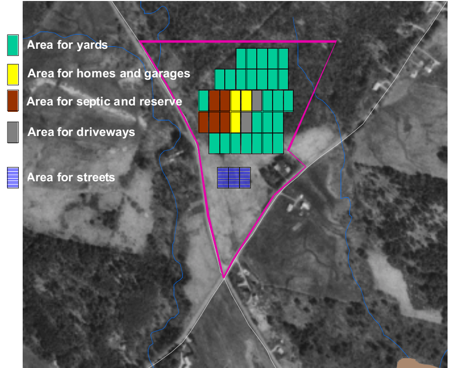
Figure 7: Land area that would be used by 35 1/2 acre lots, and the part of the 35 lots that would actually be occupied by building footprints, driveways, septic systems and streets.
