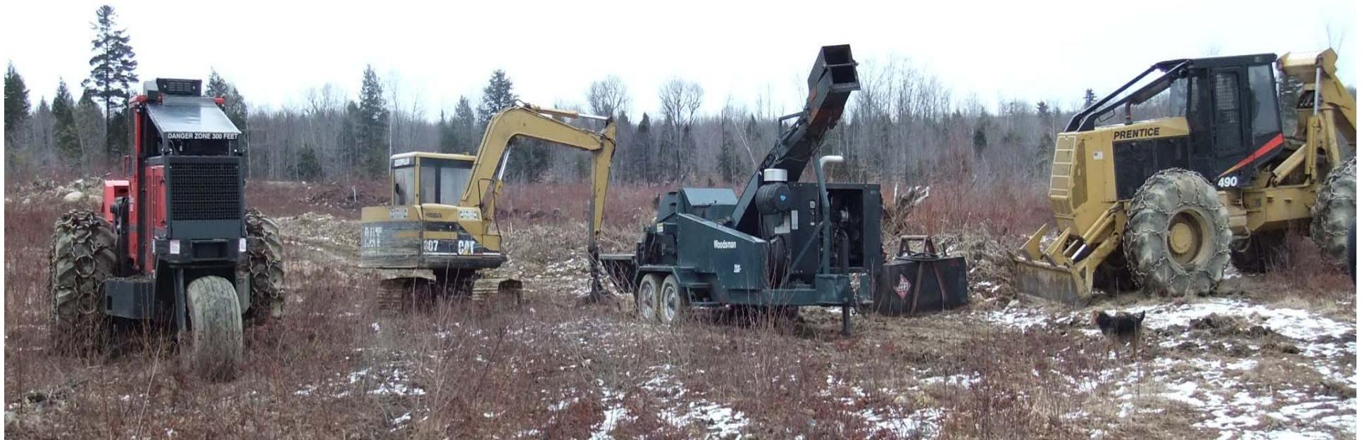
Feller-buncher; excavator; chipper; skidder
