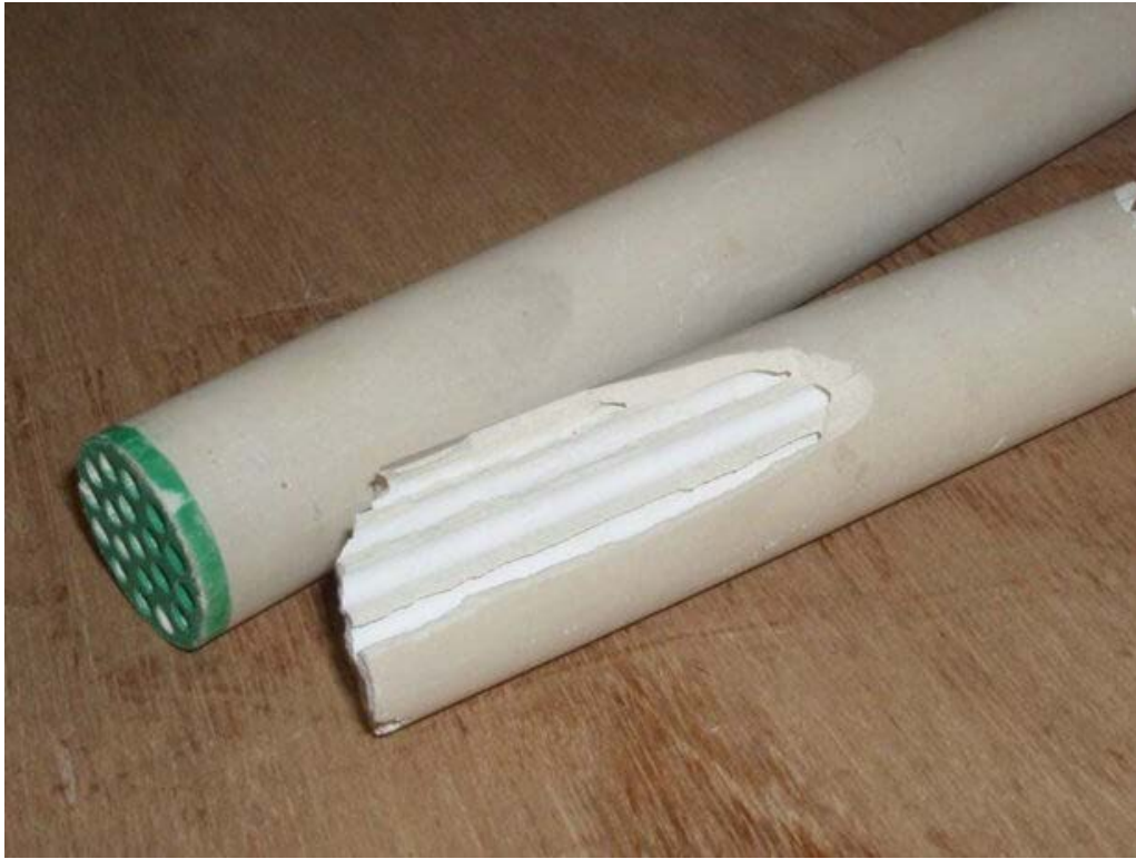
Figure 1. Ceramic UF Membrane Image Credit | Wikiwayman [CC BY-SA]
