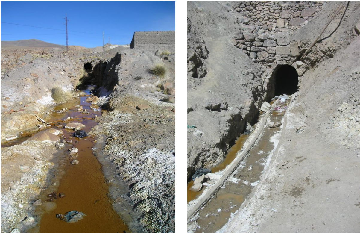
Figure 2. AMD sources 1 (left) and 8 (right). Source 1 is an abandoned mine near the eastern base of Cerro Rico. Source 8 is a functioning mine on the north slope of Cerro Rico.
