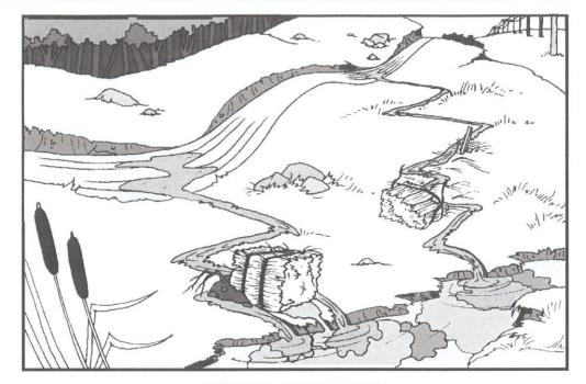
IMPROPER INSTALLATION • Hay bales are not staked • Not enough hay bales to adequately capture and slow flow • Too far from source of runoff and sediment • Improper orientation of bales: horizontal grass fibers do not provide adequate filtration • Baling twine in contact with ground
