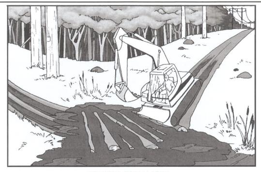
IMPROPER INSTALLATION • Area is too wet for proper application of corduroy • Insufficient corduroy to support equipment • Corduroy is sunken into wetland soil • Approaches are steep, rutted, and are not protected with additional corduroy or mats
