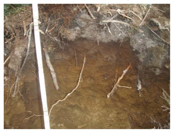
**Photograph Six.** A close up of cryic soils with thixotropic conditions. These soils have a thick elluvial layer over spodic horizons with thixotropic properties over dense basal till and bedrock.
