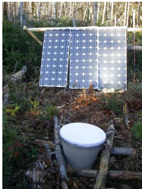
Photo 27. Acoustical monitoring stations with microphone and solar panel array.
