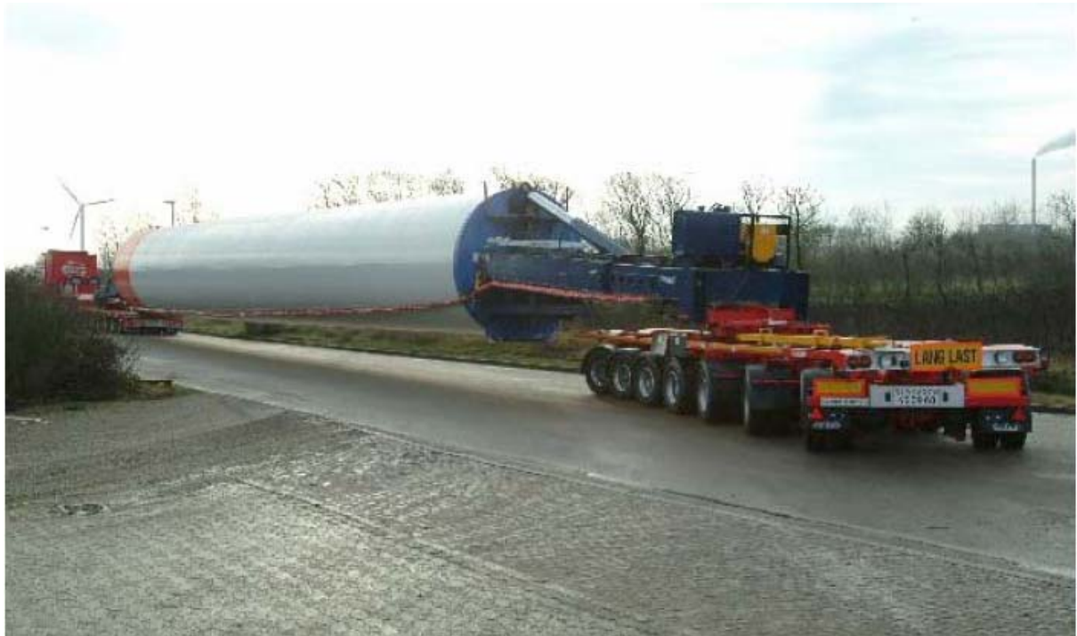
Tower section on the “New Lift adapter”
