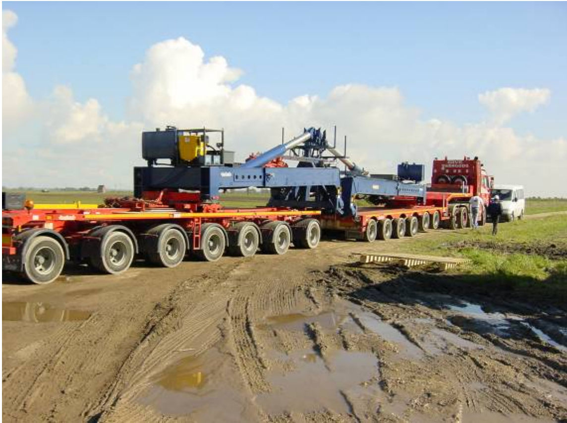
The unloaded nacelle lift adapter ready for return shipment - Total weight: 52000kg
