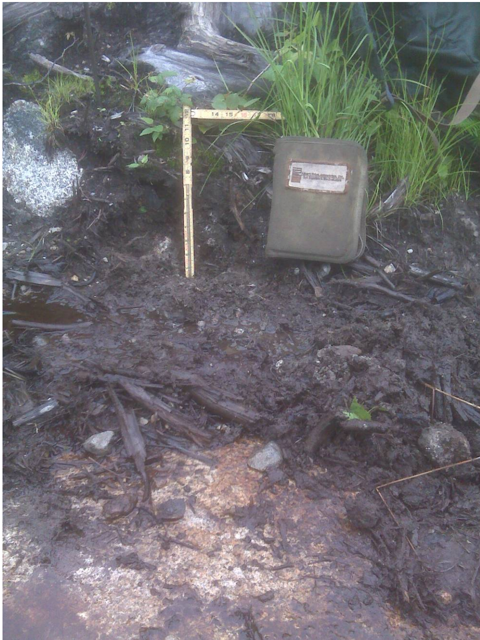
Photo 16: Test Pit 114 Abram , shallow to bedrock sandy loam soil overlying bedrock less than 10 inches in depth.
