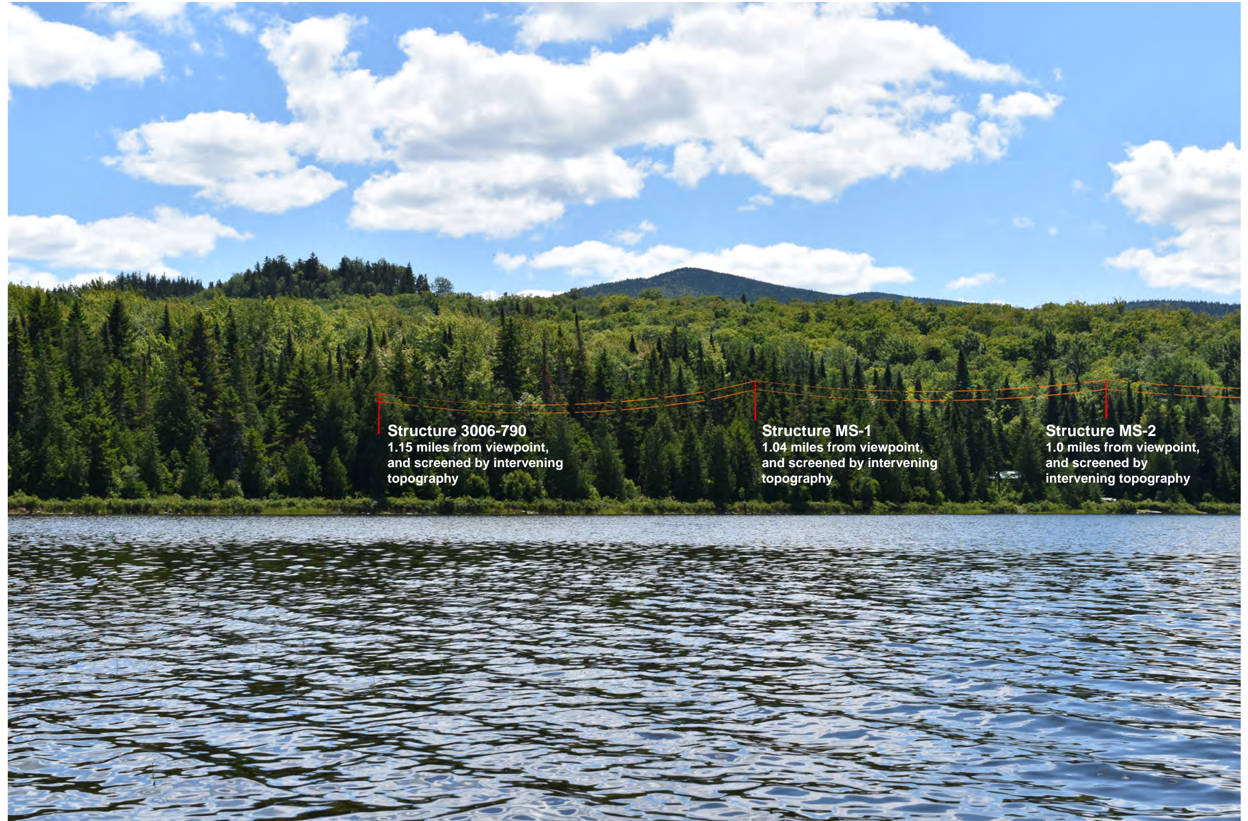
3D Model Illustration: Normal view looking southeast from the northern end of Beattie Pond toward the proposed Merrill Strip Twp alternative of the HVDC transmission line. Based on the alternative location, no structures, conductors, or shield wires would be visible from the Pond due to intervening topography.
