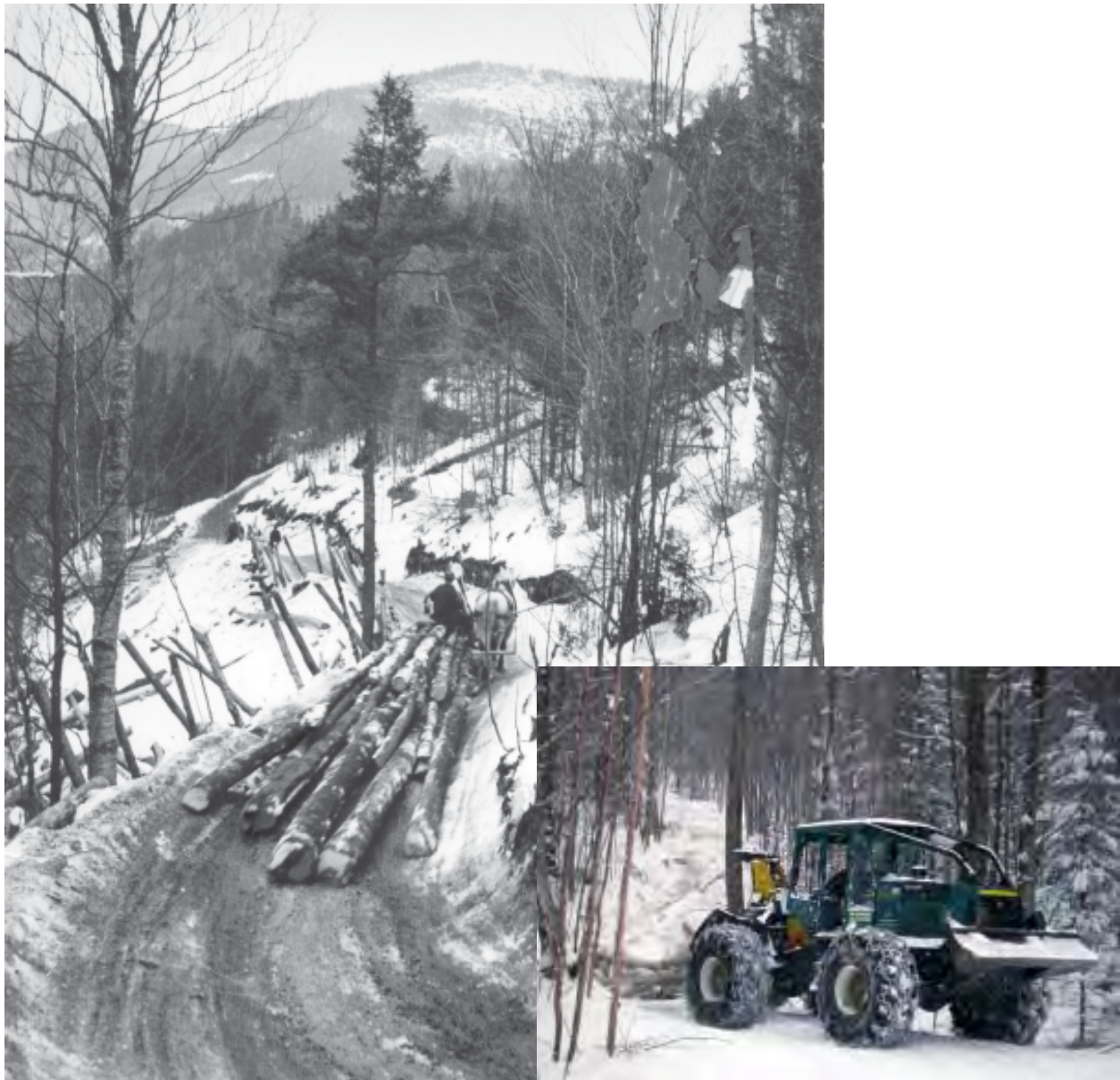
Log skidding then and now: horses drag logs at Waterville Valley ca. 1938; at right, a modern skidder at the Clear Brook timber sale. (WMNF photos by Bluford W. Muir, Forrest Seavey)
