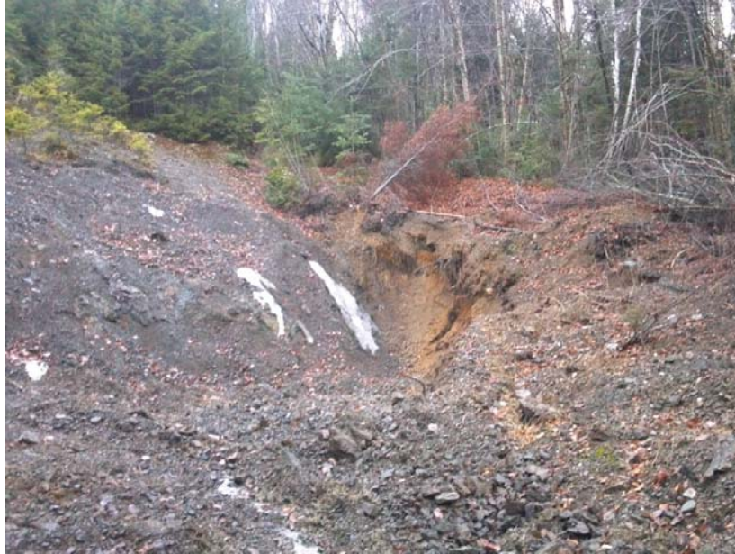
5. Example of Telos-Eliotsville-Monson soil map unit. Shallow to bedrock soils on left grade into glacial lodgement tills on right.
