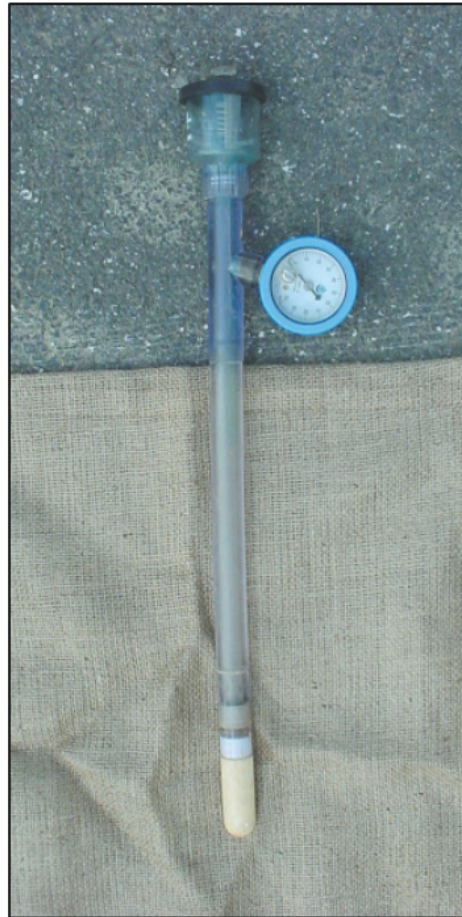
Tensiometer measures soil tension.
