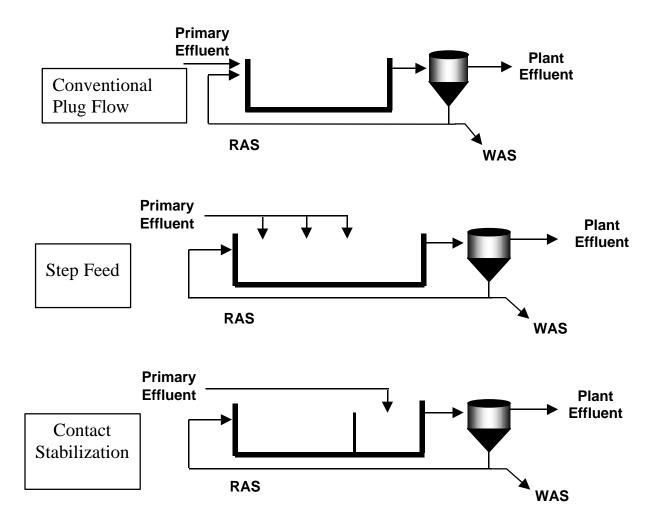
Figure 2.8 Activated Sludge Operating Modes
