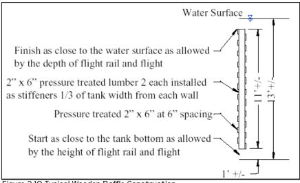
Figure 2.10 Typical Wooden Baffle Construction
