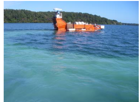
A barge applying aluminum on a lake. (Photo: WRS, Inc.)
