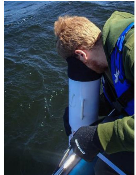
Collecting Secchi disk transparency readings on East Pond. (Photo: Logan Parker)
