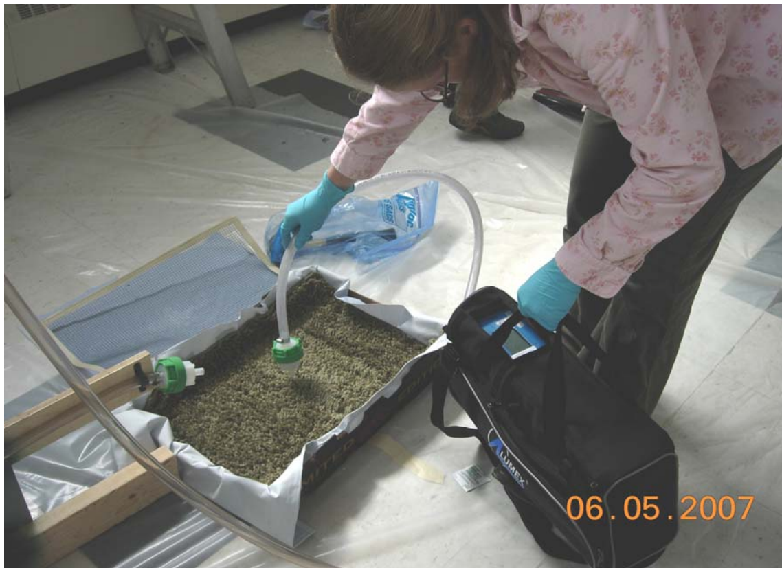
Figure B-3. Taking near-surface mercury measurements.
