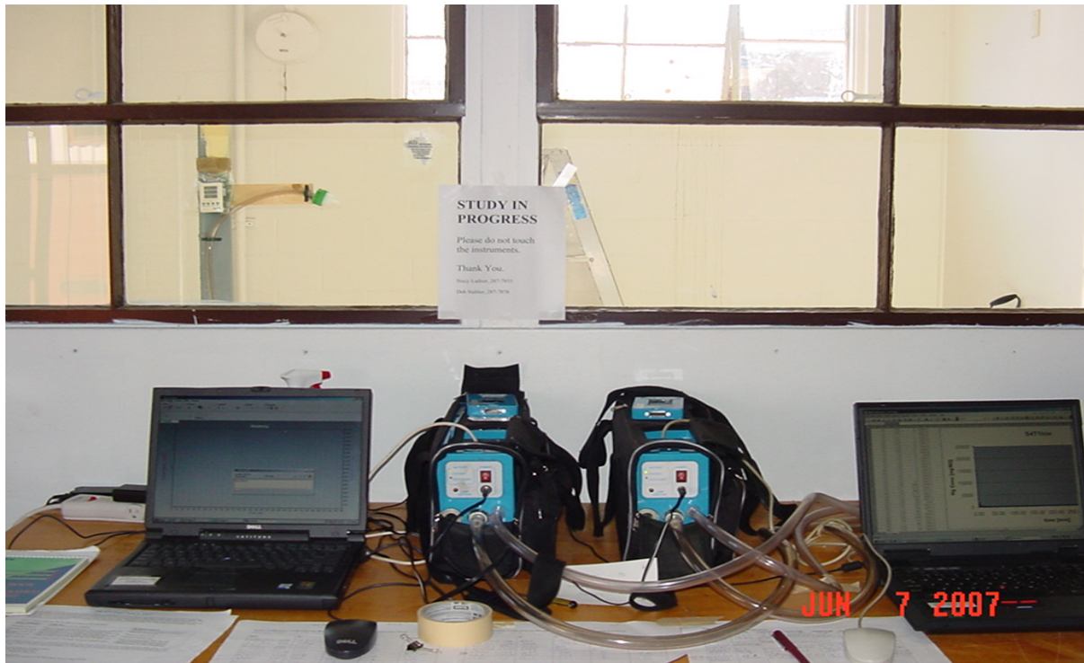
Figure 5-4. Lumex RA 915+ mercury analyzers connected to laptops
