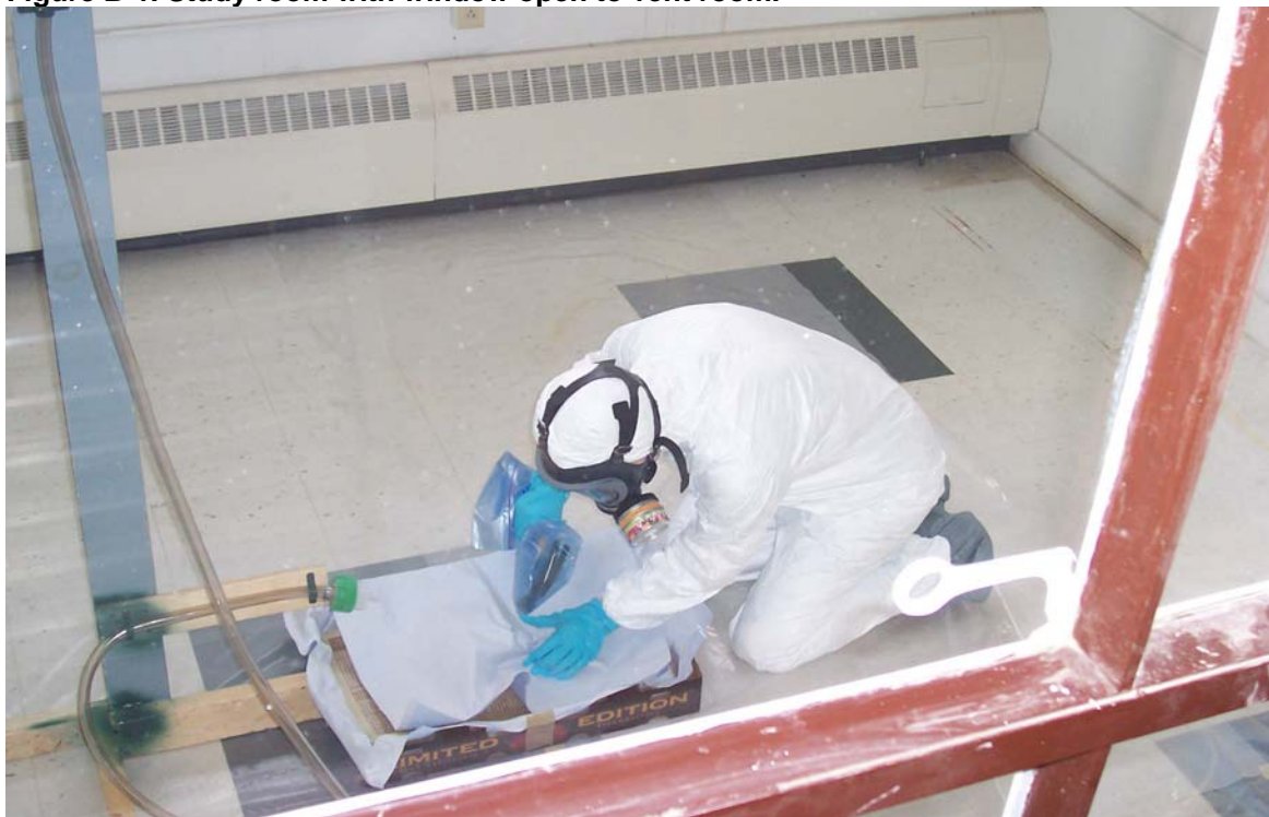
Figure B-2. Breaking a CFL.
