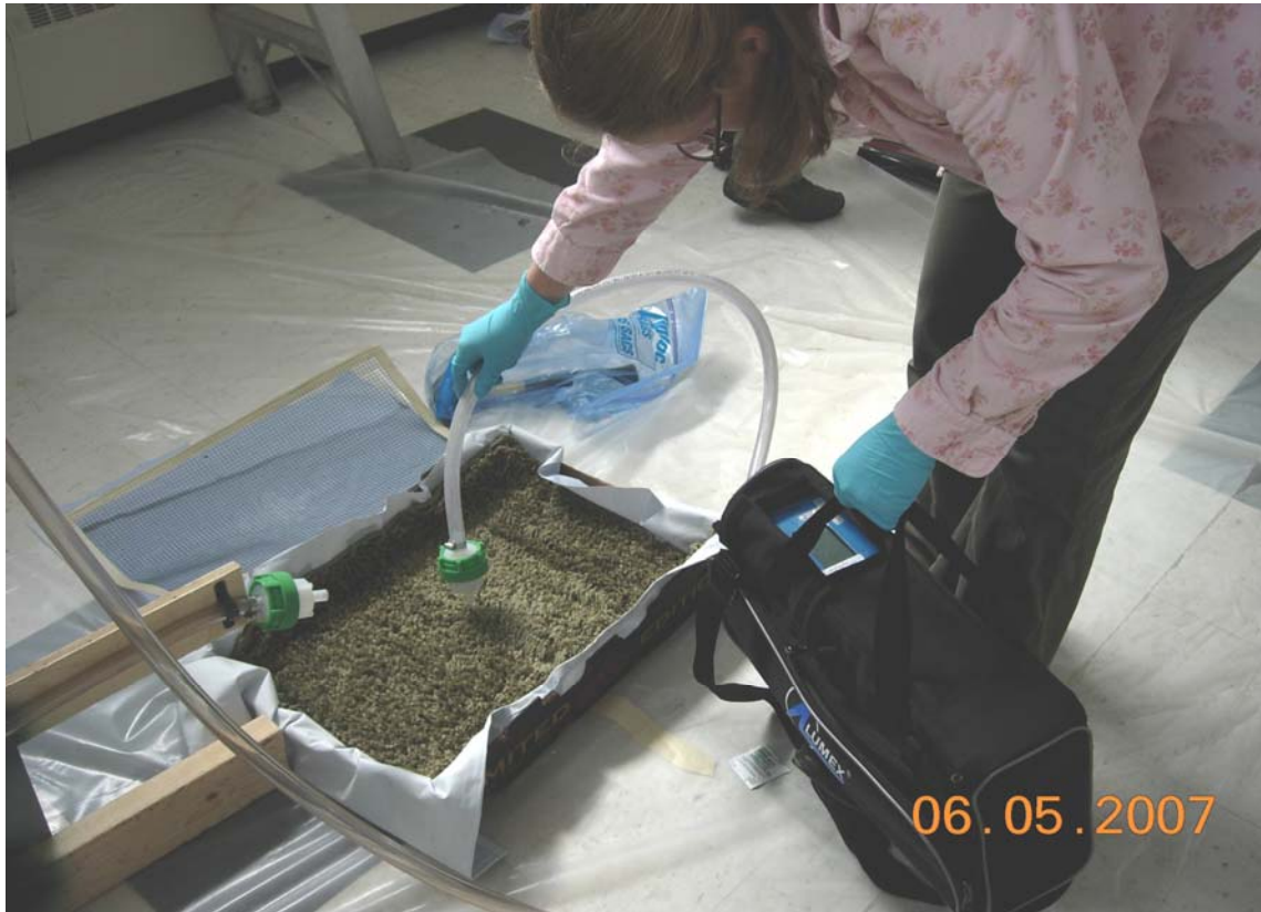
Figure B-3. Taking near-surface mercury measurements.
