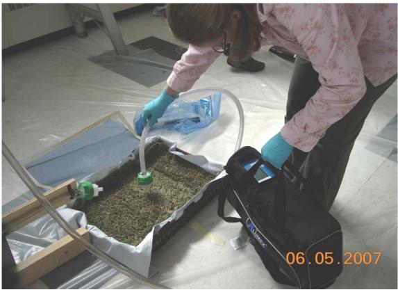
Figure B-3. Taking near-surface mercury measurements.
